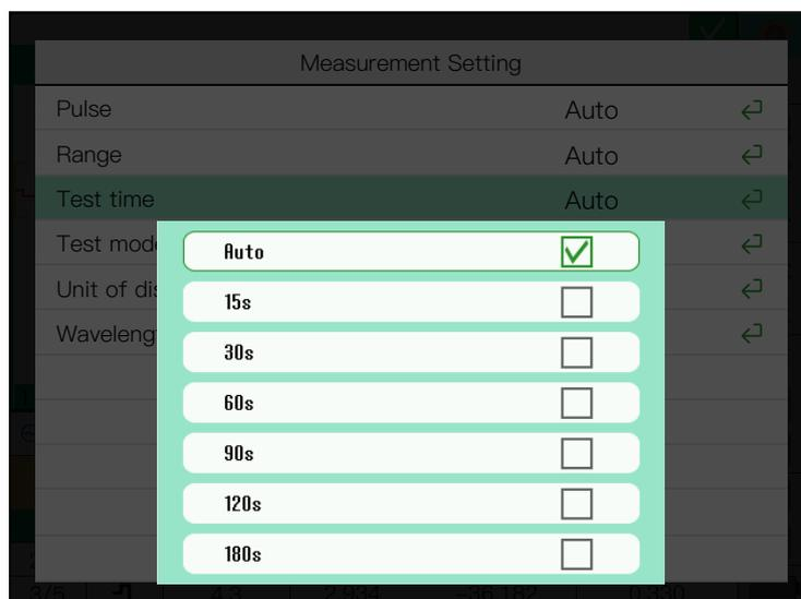
As shown in the figure above, at present, the instrument supports six test time settings: Auto, 15s, 30s, 60s, 90s, 120s, 180s, and L, of which auto defaults to 15s.
