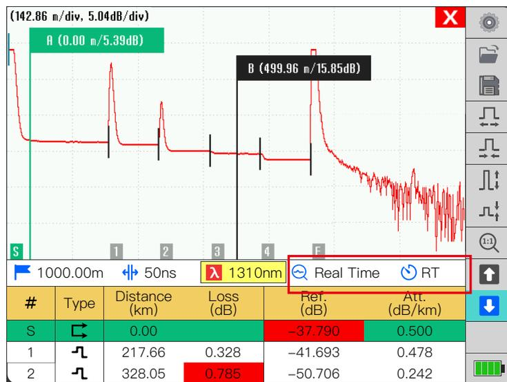
Average mode, OTDR test will use average mode to measure in order to obtain higher signal-to-noise ratio and higher small event detection ability; The average duration is set according to the needs of users. Generally, under the same test conditions, the longer the average duration, the better the signal-to-noise ratio will be. However, when the average duration is more than 3 minutes, the signal-to-noise ratio changes very little, so in the duration setting, the maximum is 3 minutes.
