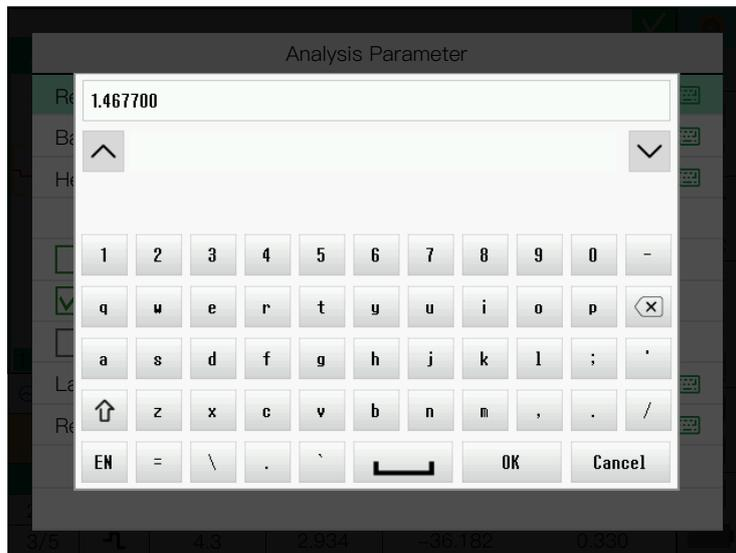
In the dual-wavelength test, only one refractive index with a wavelength of 1310nm needs to be set, and the other one will automatically calculate its refractive index according to the refractive index of 1310nm, so as to prevent a big error in the test results of the two wavelengths.
