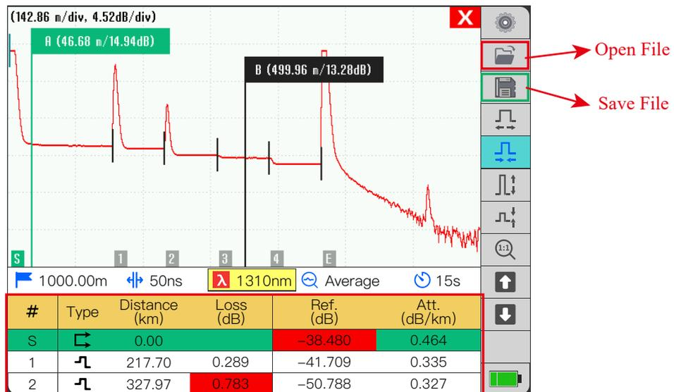
Open file: the file in the list can be opened by clicking the enter key, and the OTDR test curve corresponding to the current file will be displayed on the OTDR main interface.
