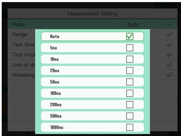
Select the required pulse width by controlling the up and down direction buttons of pulse width, press the enter button to successfully set it, and exit the pop-up window.
