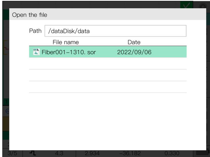
Save file: save the curve of current OTDR main interface test. Supports SOR and PDF files. Click enter to save, and the corresponding file will be saved to the set default path. If the file is saved successfully, the pop-up window of "Save the file successfully" will appear.
