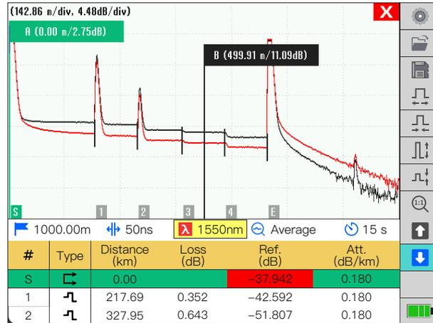
**Note:** The macro-bending event will only appear during the dual-wavelength test, so you must use the dual-wavelength test if you want to test the macro-bending event. For QX55-P SM-LIVE mode, support online testing with 1625nm; The test mode has only one wavelength and cannot distinguish the macro bending event from the splicing loss. Only a curve displayed.
