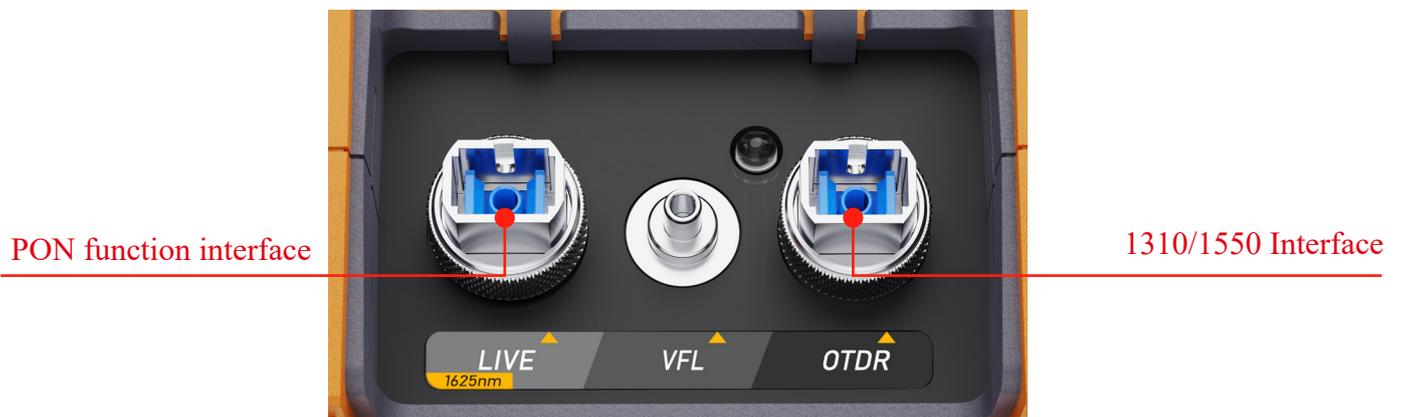
In the setting interface of OTDR, in the test setting, there is an additional SM Live option in the wavelength setting option. When this option is selected, the wavelength is switched to 1625nm, as shown in the following figure:
