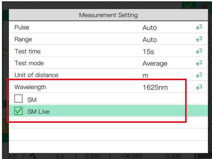
When using the 1625nm wavelength test, the wavelength switching function fails, as shown in the following figure:
