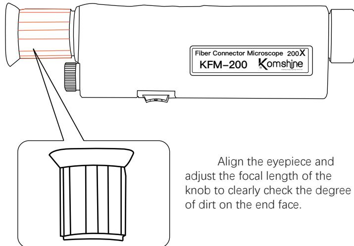
Align the eyepiece and adjust the focal length of the knob to clearly check the degree of dirt on the end face.
